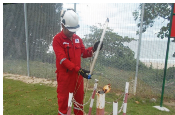
Groundwater Monitoring in progress: Bailleurs are used to purge and sample groundwater from the respective wells. Samples are contained in sampling bottles with the respective parameter's preservatives.
