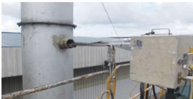
Dust particulate sampling for stack emission at LCOT using the ESC A-2000 Automated Isokinetic System
